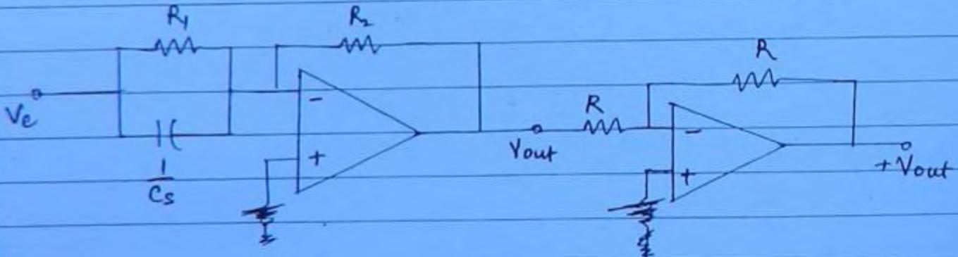
$$\frac{V_e - V_1}{R_1} = \frac{V_1 - V_{out}}{R_2}$$
