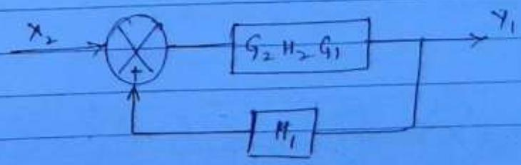
$$\frac{Y_1}{X_2} = \frac{G_2 H_2 G_1}{1 - G_1 H_1 G_2 H_2}$$
