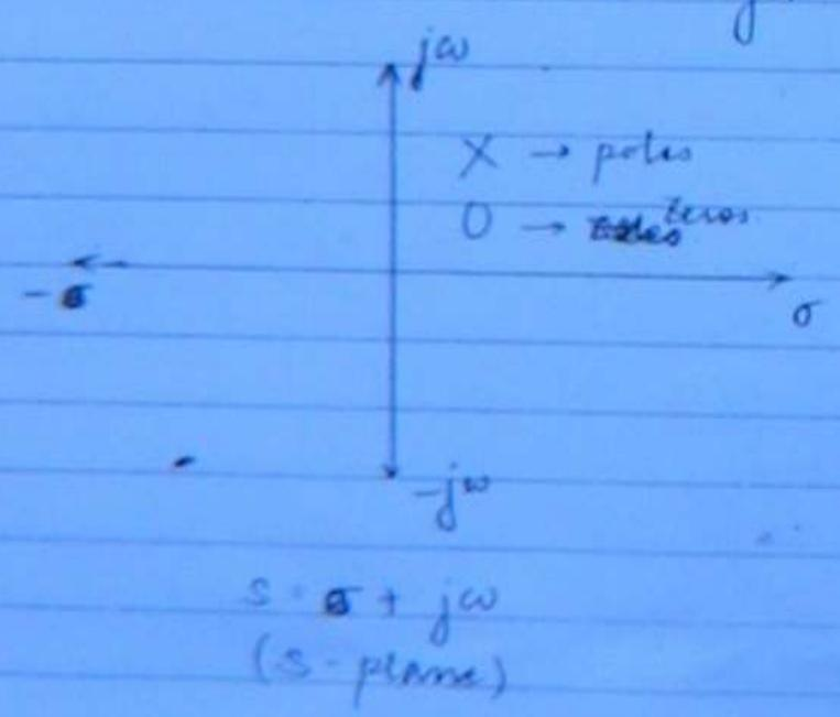
\* From eq (1), transfer function of LTI system may be defined as ratio of Laplace transform of output to Laplace transform of input under the assumption that systems initial conditions are zero.
