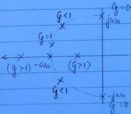
Most of the control systems are defined for  $\zeta < 1$  because the response can be analysed using more of specifications
