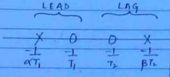
$$\angle F(j\omega) = \tan^{-1} \omega T_1 - \tan^{-1} \omega \alpha T_1 + \tan^{-1} \omega T_2 - \tan^{-1} \omega \beta T_2$$
