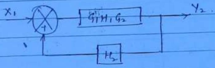
$$\frac{Y_2}{X_1} = \frac{G_1 H_1 G_2}{1 - G_1 H_1 G_2 H_2}$$
