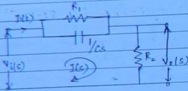
$$V_i(s) = I(s) \left[ \frac{R_1 + R_2}{R_1 C s + 1} \right]$$
