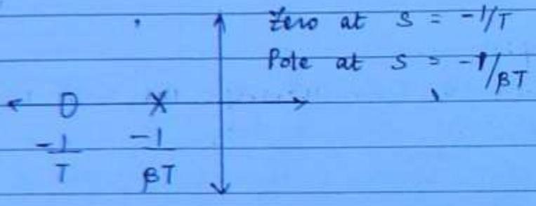
NOTE → If a pole is added to a system T.F in terms of compensation, it represents a LAG Compensator.
