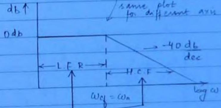
$$\text{Slope (m)} = -40 \text{ db/dec}$$
