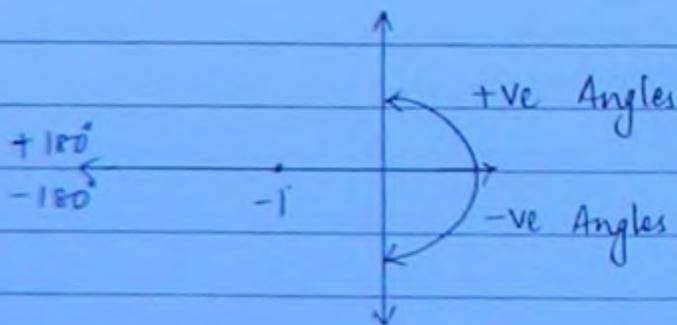
Angle condition may be stated as, for a point to lie on root locus, the angle evaluated at that point must be an odd multiple of  $\pm 180^\circ$
