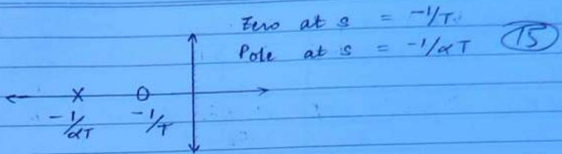
NOTE  $\rightarrow$  The frequency nearest to origin is a zero in a LEAD compensator. Therefore its effect is not dominating.
