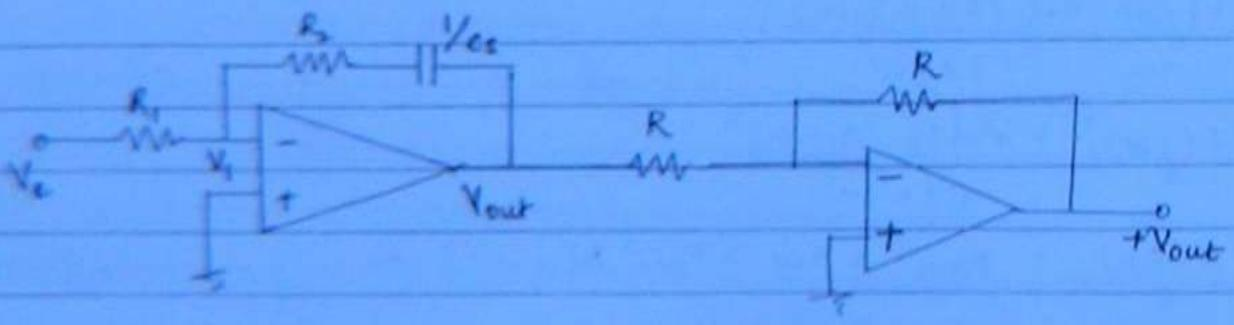
$$\frac{V_e - V_i}{R_1} = \frac{V_i - V_{out}}{\frac{R_2 Cs + 1}{Cs}}$$
