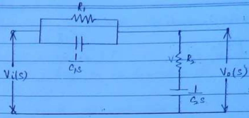
$$\frac{V_o(s)}{V_i(s)} = \frac{\alpha(1+T_1s)(1+T_2s)}{(1+\alpha T_1s)(1+\beta T_2s)}$$
