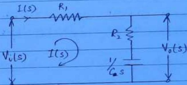
$$V_i(s) = I(s) \times \left[ R_1 + R_2 + \frac{1}{C_s} \right]$$
