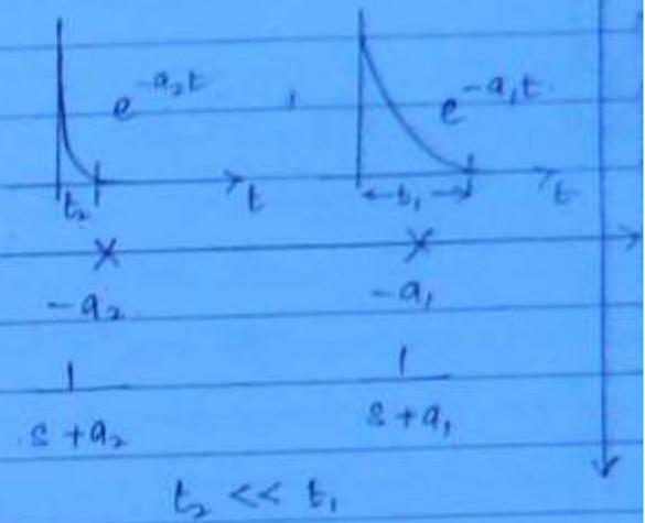
The time response of higher order system is obtained by approximating to second order system w.r.t dominant poles. The time domain specifications obtained for approximated second order system are valid for the higher order system also.
